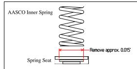
Remove approx. 0.015" (.38mm) from the seat in the area shown so the inner spring sits freely in the seat.
